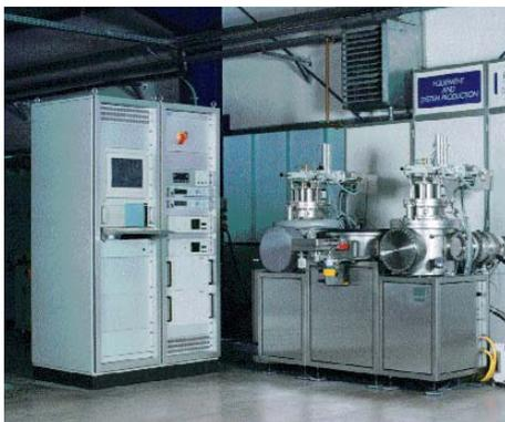
Multi chamber ECR-RIE system with automatic sample transfer system for fluorine and chlorine processes
