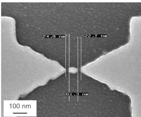
REM picture of a metal cluster between two contact tips
