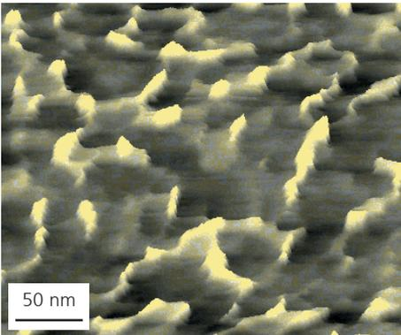
AFM picture of a surface of a titanium-platinum layer tempered at 700 °C
